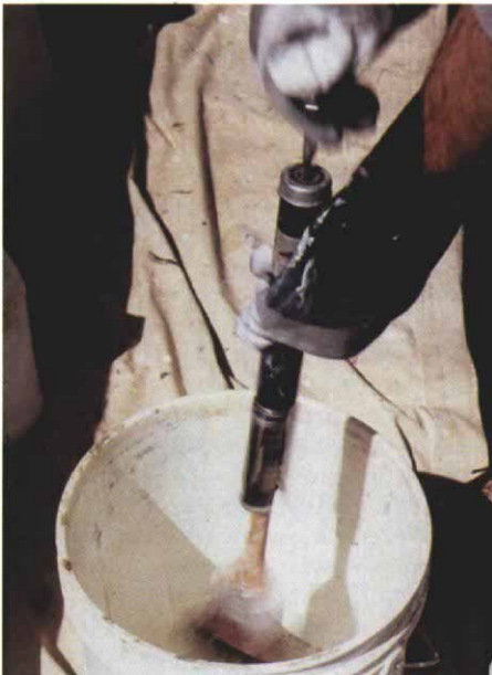
Centrifugal force flings paint and solvent off a brush or a roller cover when you use a spinner. Keep the brush or roller cover toward the bottom of the bucket when you spin it.
