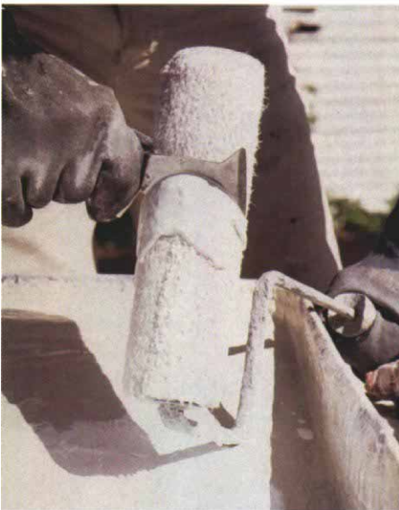
A three-in-one is handy for scraping excess paint off a roller cover. A blade on the end of the tool is good for removing partially dried paint from a paintbrush ferrule or for opening cans of paint. A three-in-one costs about $5.
