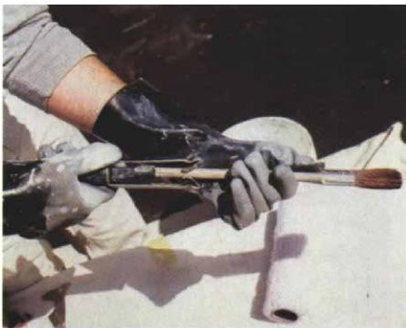
A spinner firmly holds a paintbrush in its two sets of metal tangs. A roller cover fits over the tangs for spinning. A spinner costs about $30.
